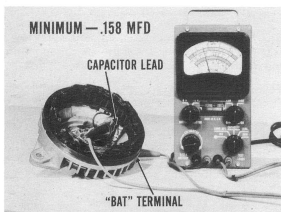
Fig. 7—Testing alternator capacitor
