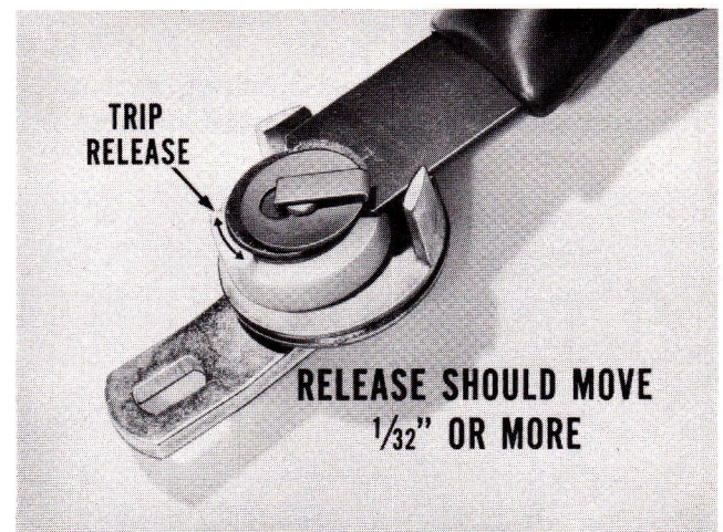
Fig. 20—Checking overtravel assembly
