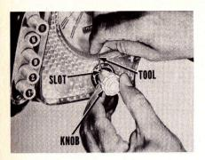
Next, turn the windshield wiper knob to the full-on position to bring the slot in the underside of the knob to the top. Then, insert a small pointed tool in the slot in the knob and apply pressure on the retaining spring. At the same time, pull the knob from the shaft.
