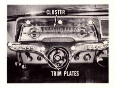
Then, work the speedometer cable up through the dash panel. At the same time, tilt the cluster outward from the panel. Tilt the cluster sufficiently to provide enough clearance to permit the speedometer cable to be disconnected from the head. Disconnect the cable.
