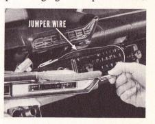
Next, disconnect the sending unit wire from the "S" terminal on the gauge. Connect one of the tester leads to the "S" terminal and the other to a good ground on the cluster.
