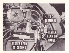
Testing Procedure—Chrysler. First, remove the jacket tube cover as outlined in "Cluster Removal". Then, disconnect the wire from the terminal of the oil pressure gauge marked "S". Connect one tester lead to this terminal. Connect the other tester lead to a good ground.
