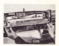
Caution: Care should be exercised not to remove the bezel and dial from the cluster housing. The panelescent lighting, composed of a number of small panelescent lamps, should not be disturbed. Special fixtures are required to assemble the lamps and, therefore, the speed-ometer head and housing should be serviced as an assembly only by the speedometer manufacturers' service dealer.
