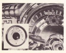
The last test is to move the pointer to the "H" position on the tester. The gauge needle should register at the "F" position, or within  $\frac{3}{32}$  inch either side of it.
