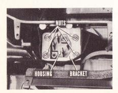
Working through the cluster opening in the housings, remove the four nuts which secure the pushbutton selector housing to the mounting bracket. Then, move the selector housing back away from the bracket.
