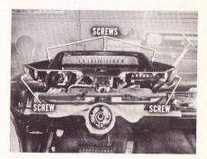
Raise the upper speedometer housing, speedometer head, and the two bezels (if attached) as a unit until it clears the lower housing.
