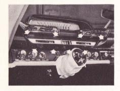
From the underside of the front face of the instrument cluster, remove the two rows of four attaching screws. Next, reach under the instrument panel and loosen the five wiring harness clips to provide more flexibility for the harness.
