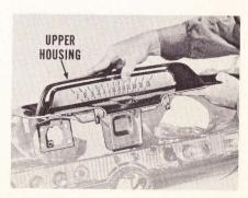
Chrysler—The gauges and speedometer head on these models are contained in a single cluster. The gauge cluster must be removed before the speedometer head can be removed. The steering wheel must be removed to remove the gauge cluster or the speedometer head.
