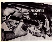
cable up through the dash panel until the cluster can be tilted out far enough to permit disengaging the speedometer cable from the head. Disconnect the speedometer cable. Place a cloth along the lower edge of the instrument panel cluster opening to insulate the cluster, and lay the cluster against the steering column to test the gauges.
