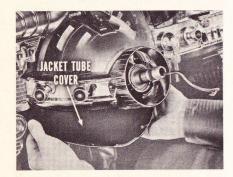
Working from under the steering column, remove the six screws which attach the cover to the underside of the steering gear jacket tube, and remove the cover.
