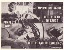
before connecting the tester. Reach up under the instrument panel and disconnect the purple wire from the terminal on the temperature gauge. Connect one lead of the tester to the terminal from which the wire was disconnected. Then, connect the other tester lead to a good ground.
