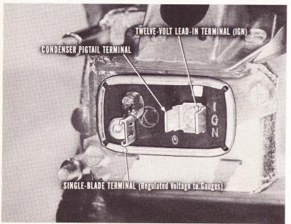
nals and a single-blade terminal mounted on its base. The twelve-volt lead-in is connected to one of the double-blade terminals marked "IGN". The other blade carries the condenser pigtail. The condenser is connected in the circuit to eliminate noise in the radio that might be set up by the vibrating contacts in the regulator. The single-blade terminal is for the wires which carry the regulated voltage to the various gauges.
