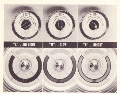
the light to glow in full brilliance. A dim light with the pointer at "H" would mean there is resistance in the wiring.
