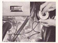
However, if the gauge does not register, it can be assumed the sending unit is all right, but there may be difficulty in the wiring or the gauge. The wiring should be traced out for chafed and grounded areas, poor connections, or breaks in the wire.
