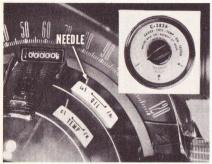
Place the pointer on the tester in the "L" position, and turn the ignition "ON". The oil pressure gauge needle should show at the "LO" position on the scale.
