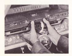
Then, tilt the cluster down and disengage the overlap at the center of the cluster. Carefully pull the cluster from the panel and rest it on the protected steering column to test the gauges.
