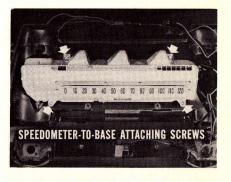
Extreme care should be exercised when installing the speedometer head not to kink the outer casing of the speedometer cable which might cause noise.
