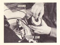
Turn the ignition "ON". Then, move the pointer on the tester to the "L" position and the needle on the gauge should show "E". Continue the test by moving the pointer to "M", and the gauge needle should slowly move to the halfway position on the dial.
