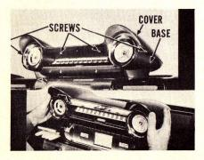
To remove the cluster, first remove the four screws from the upper edge of the speedometer cover base which secure the cover to the base. Due to the limited space between the windshield and the left end of the cover base, an offset Phillips screwdriver should be used to remove the
