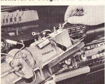
the wiring from all gauges and separate the lamp bulb sockets from the cluster. Then, place the cluster on a padded or otherwise protected area of the workbench to guard against scratching it. The gauge can then be removed from the cluster by removing the two attaching screws.
