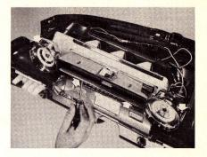
Next, remove the four speedometer-to-base attaching screws and raise the speedometer head, being careful not to damage the cable. Then, disconnect the cable from the speedometer head.
