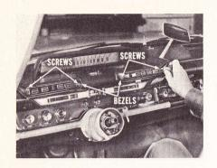
Remove the two screws from each of the two pushbutton bezels and carefully remove the bezels to avoid chipping the finish. Then, carefully remove the cluster.
