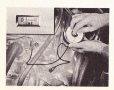
Next, turn the pointer to "M" and the gauge needle should slowly move to the middle of the scale. Here, again, the 1/8-inch tolerance either side of the mid-position of the scale is in order.
