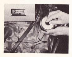
Set the pointer on the tester on "L". Turn the ignition key "ON" and the gauge needle should be at the "C" or cold position. If the needle varies less than ½ inch either way from the "C" position, the gauge can be considered to be functioning satisfactorily. If the variation is greater than ½ inch, the gauge is inaccurate and should be replaced.
