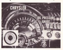
If the gauge does not register, or registers improperly, it can be assumed that the sending unit is okay, and the wiring from the sending unit to the gauge, or the gauge itself, is at fault. Further tests should be made at the gauge.
