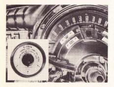
In the second test, move the pointer to the "M" position and the needle should slowly move to the halfway position on the gauge, or within  $\frac{1}{16}$  inch either side of it.
