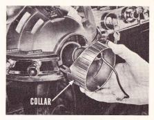
Reach up under the instrument panel and remove the two long screws and spacers which attach the cluster to the support. These screws are located just behind the steering tube collar attaching screws.
