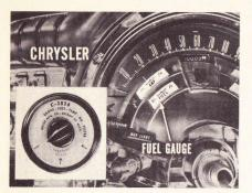
Start the test by first turning the ignition "ON". Then, move the tester pointer to the "L" position and the gauge needle should stay at the "E" position on the scale, or within  $\frac{3}{32}$  inch either side of it. This tolerance permits a small reserve of fuel in the tank when the needle is at the "E" position.
