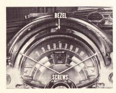
Remove the two screws which secure the bezel to the instrument panel, and remove the bezel.
