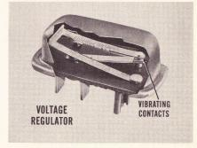
When testing at the gauge, extreme care must be taken not to connect twelve volts directly from the battery to the gauges. The twelve-volt battery voltage must be connected through the regulator.
