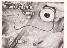
wire from the sending unit. Then, connect one lead of the tester to that wire. Connect the other tester lead to a good ground. This removes the sending unit from the circuit and the tester takes its place.
