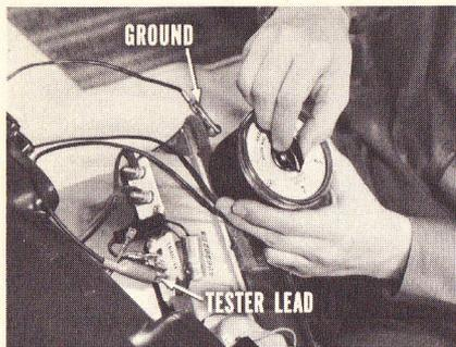
Turn the ignition "ON". Then, move the pointer on the tester to the "L" position and the needle on the gauge should show "E". Continue the test by moving the pointer to "M", and the gauge needle should slowly move to the halfway position on the dial.
