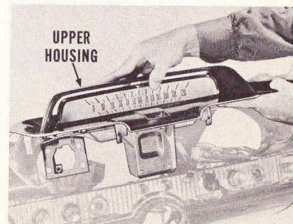
**Chrysler**—The gauges and speedometer head on these models are contained in a single cluster. The gauge cluster must be removed before the speedometer head can be removed. The steering wheel must be removed to remove the gauge cluster or the speedometer head.
