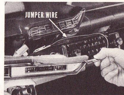
Next, disconnect the sending unit wire from the “S” terminal on the gauge. Connect one of the tester leads to the “S” terminal and the other to a good ground on the cluster.
