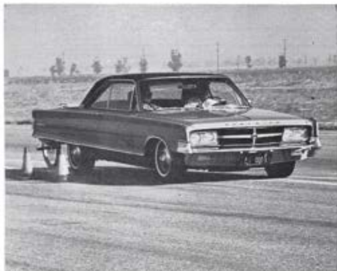
The 300-L is one of few large cars that have adequate brakes. Panic stops were short, considering the 2.5-ton test weight.
