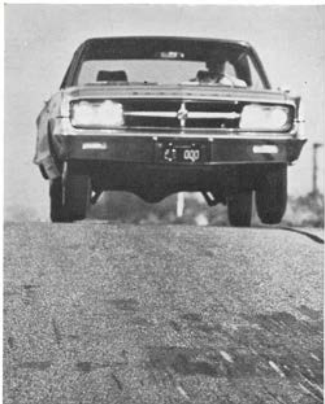
She flies through the air with the greatest of ease—and she doesn't bottom on impact; another benefit of stiff springing.
