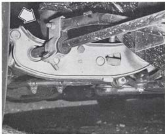
Rubber stop (arrow) contacts lower member early in upward travel, gives variable rate and good snubbing to front suspension.
