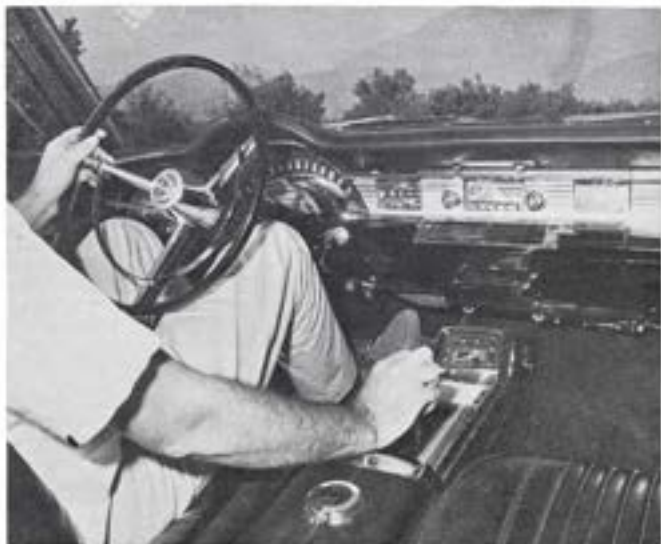
Well located selector and vacuum gauge are standard with automatic trans. Tach replaces gauge with optional four-speed box.
